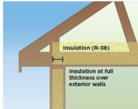
An "energy truss" can prevent cold corners by allowing the ceiling insulation to overlap with the wall insulation
